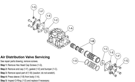
**Step 8:** Reassemble in reverse order, starting with step 3.
