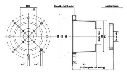
The auxiliary flange, if specified, is supplied already fitted to the bell housing .
